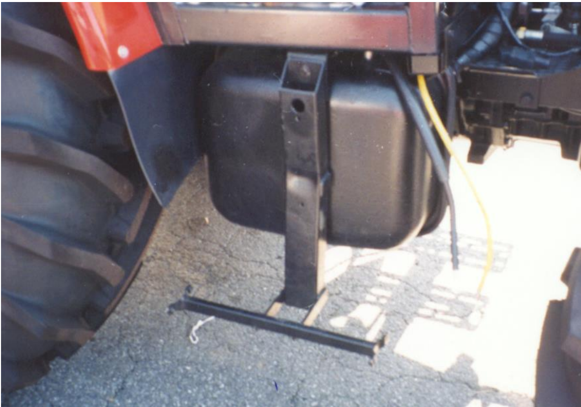
Battery box support frame (existing from step assembly).
