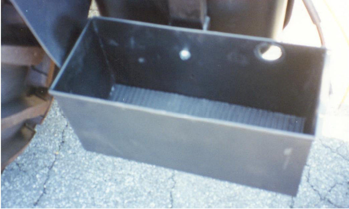
Battery box in place on frame.
