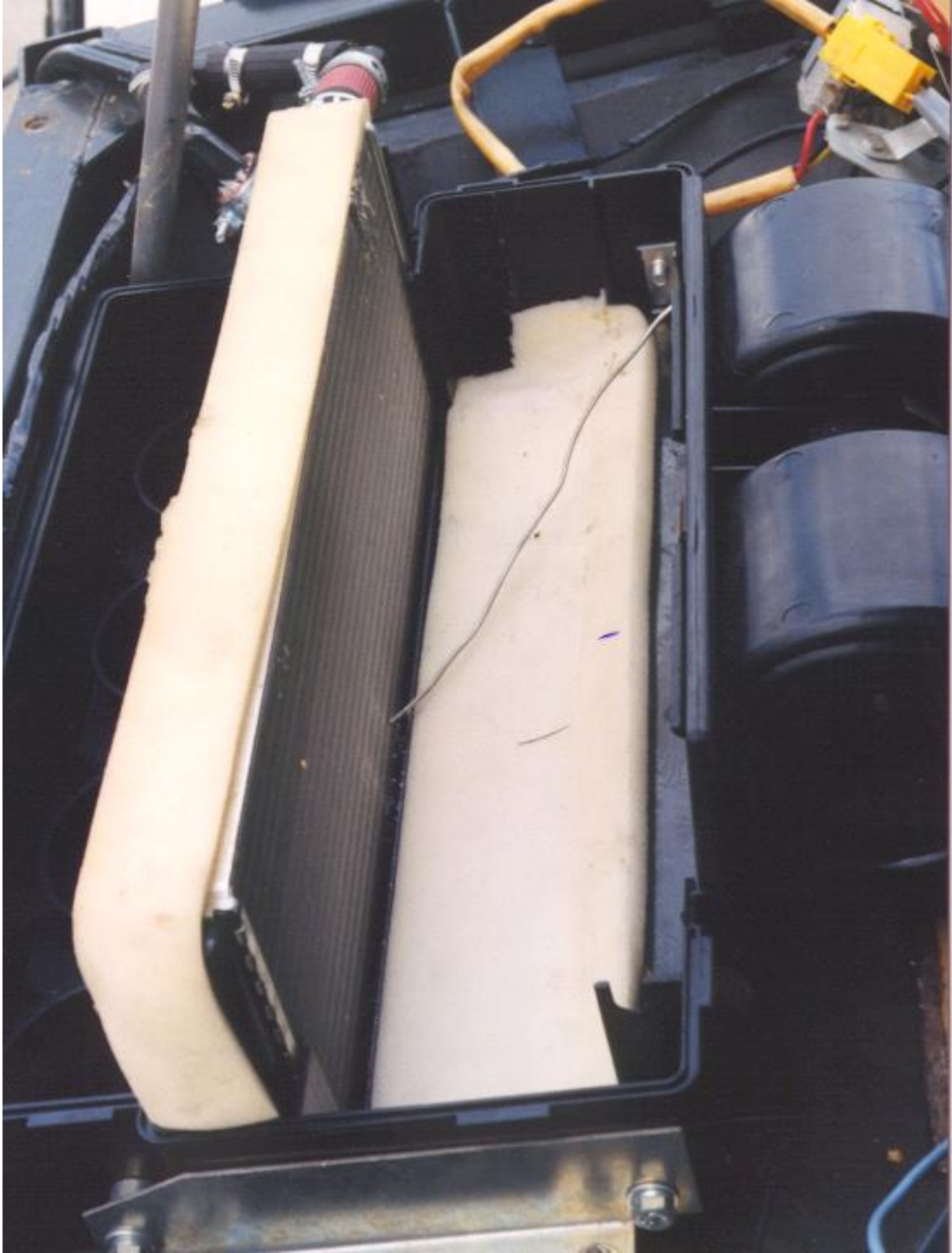
Open evaporator heater box showing heater core in place.
