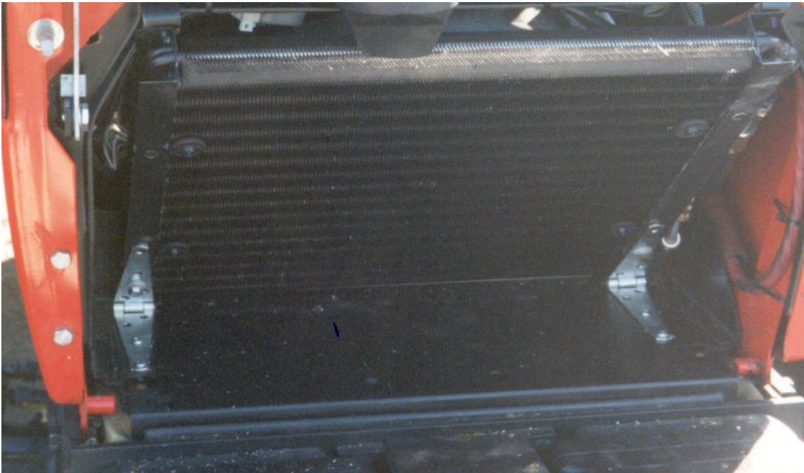
Condenser in place showing lower brackets (hinges).
