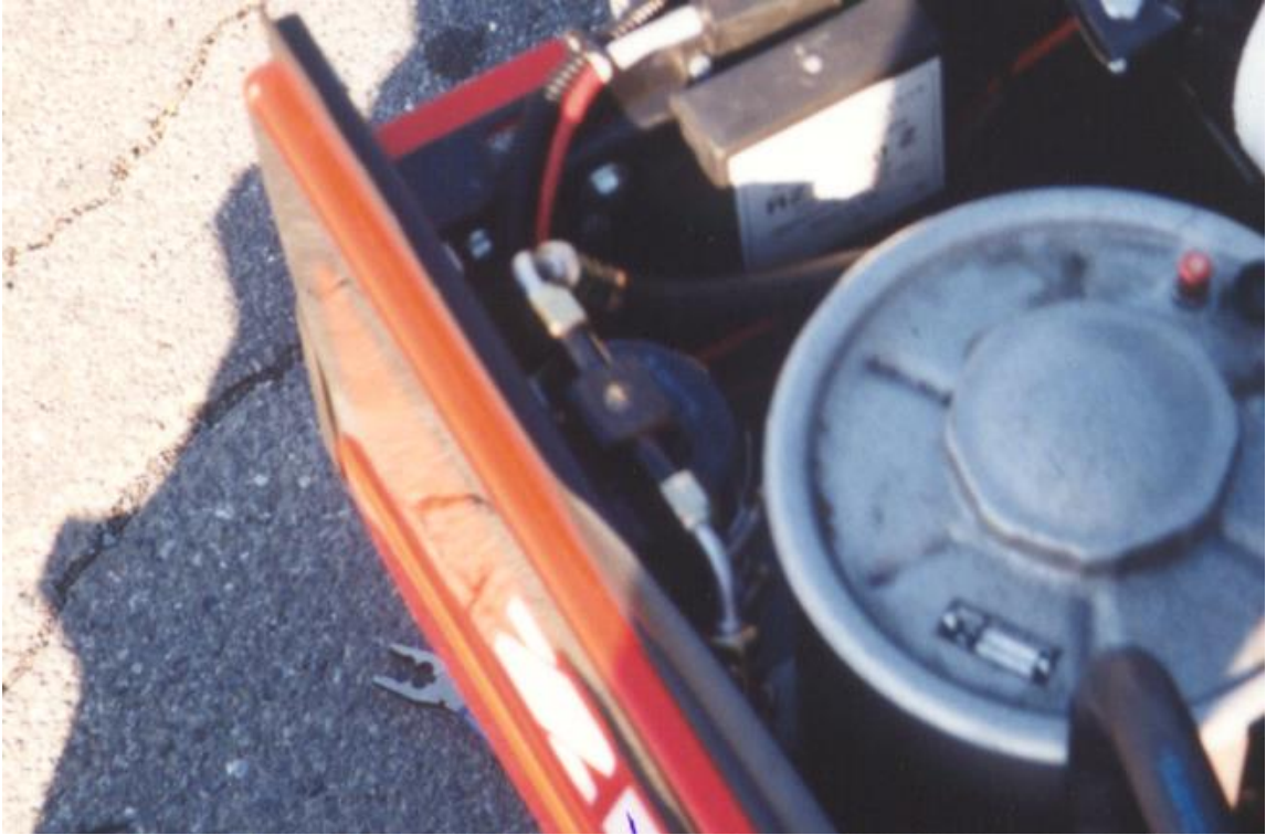
Receiver drier in place viewed from top.
